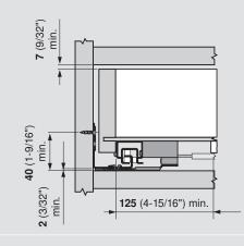
**NOTE:** MOVENTO runners will sit **2** (3/32") higher when using the lateral stabilizer in bottom mount applications and may have to be raised for some bottom mount drawer applications using SERVO-DRIVE
