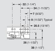
NOTE: Elongated holes are for ±4.5 (3/16") depth adjustment only. Additional screws must be used to secure the runner to the cabinet.
