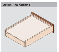
Make the back panel shorter and extend the drawer bottom to the back of the drawer
