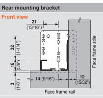
NOTE: For frame applications, use a minimum of three screws per bracket
