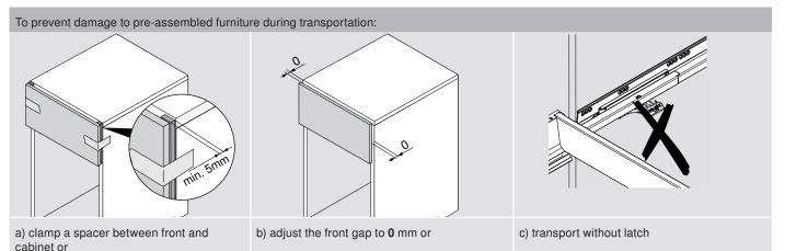
NOTE: Front gap will have to be readjusted during installation
