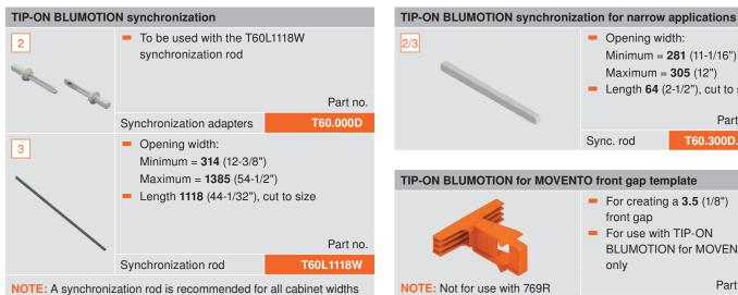
NOTE: A synchronization rod is recommended for all cabinet widths for optimal function
