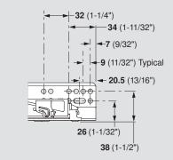
NOTE: Elongated holes are for ±4.5 (3/16") depth adjustment only. Additional screws must be used to secure the runner to the cabinet.
