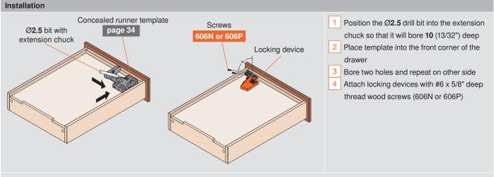
**NOTE:** The mounting screws must go in at a precise angle and the locking device must fit flush to the drawer bottom to ensure proper function of the complete drawer system
