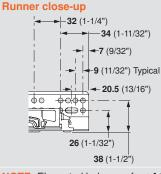
**NOTE:** Elongated holes are for  $\pm$ **4.5** (3/16") depth adjustment only. Additional screws must be used to secure the runner to the cabinet.
