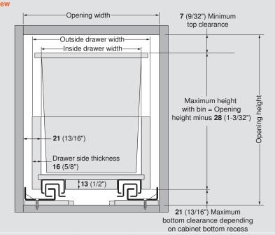
**NOTE:** Drawer side material thickness may vary. Precise measurement of drawer side material thickness should be used when calculating outside drawer width using the table below. Inside drawer width **must** equal opening width minus **42** (1-21/32") for MOVENTO runners to align and function optimally.
