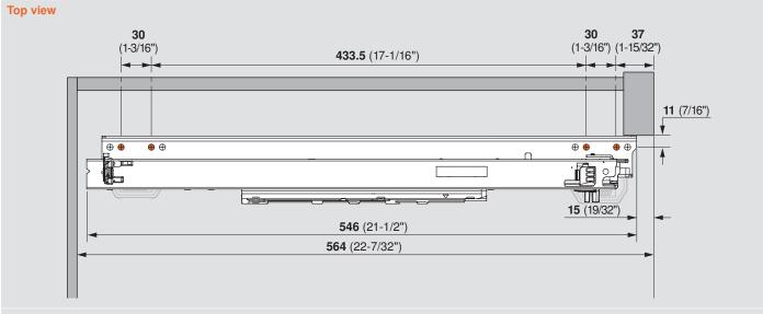
NOTE: Orange dots indicate pre-mounted screw locations. All four are required to meet specified load capacities.
